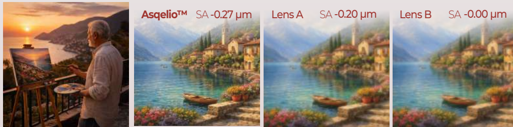
Simulation generated using Zemax OpticStudio 18.9 for a 6 mm pupil diameter considering the average human cornea of +0.27 \mu\text{m} SA.
